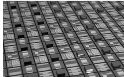
Fig. 3. Dummy MEMS chips flipped and bonded to a substrate wafer with Au stud bumps. No underfill was included.
