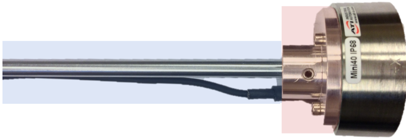
Figure 4.6: ATI Mini40 IP68 sensor mounted to the rod (blue) via the connector plate(red).
