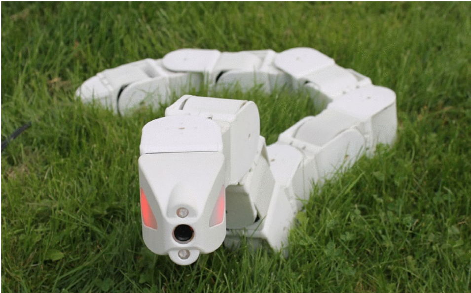
Figure 1.3: Mamba [32] on land.
