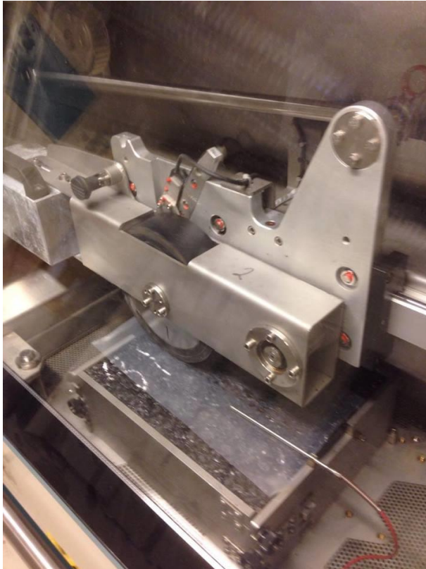
FIGURE 16 Asphalt specimen being tested in a wheel-tracking device
