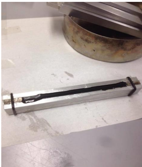
FIGURE 14 A finished molded sample of bitumen ready for trimming
