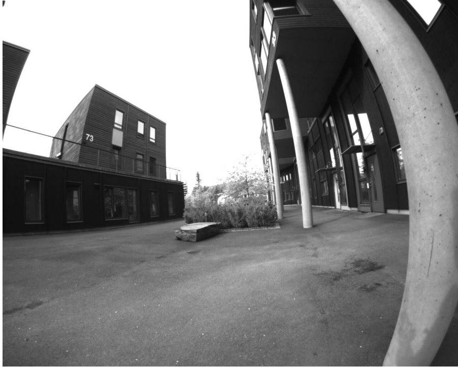
Figure 7.4: Image taken with the IDS camera. Heavy distortion resulting from the wide-angle lens.
