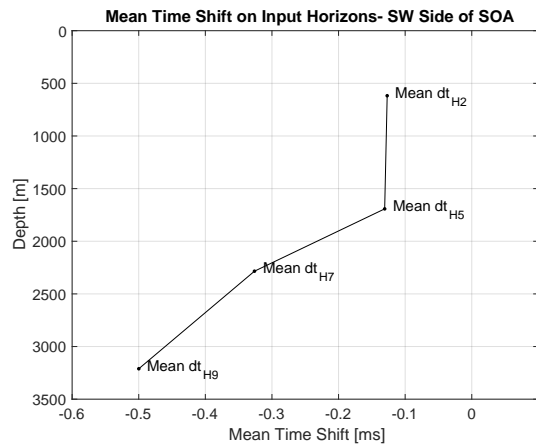
Figure 4.28: Input seismic horizons and corresponding average time shift from SW-side of SOA
