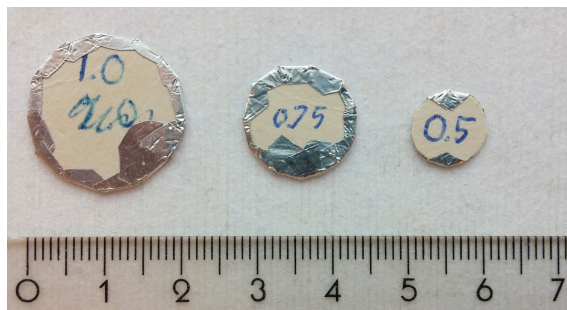
Fig. 5. Back sides of pads made from aluminum tape wrapped around to the backside of cardboard discs, with total thickness of 0.65 mm. The front sides are covered by one layer of aluminum tape. The ruler scale is in cm.
