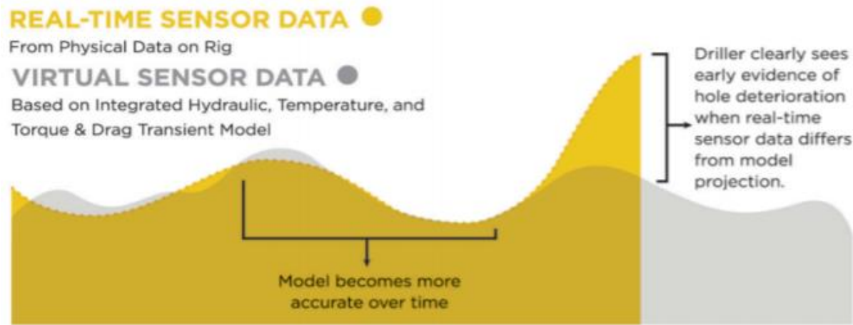
Figure 2.1: The principle behind IRIS' model, which compares real-time sensor data with calculated model data (Chmela et al.).
