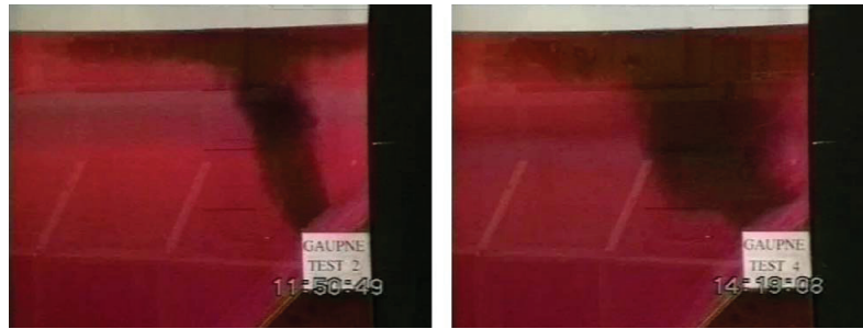
Fig. 6. Side views of the simulated fresh water plumes (dyed black) in the stratified recipient with (right) and without (left) a diffuser plate over the outlet.
