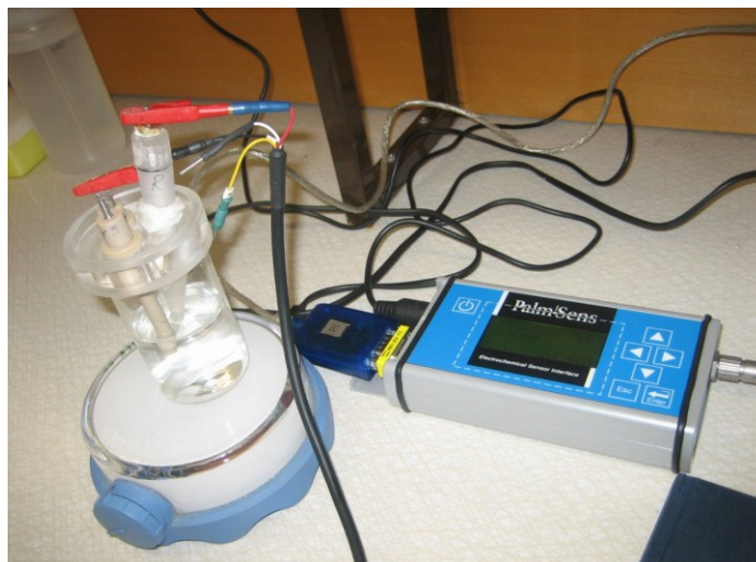
Figure 13 The overview of PalmSens PC connecting with three electrodes: reference electrode, counter electrode and working electrode respectively. (Photo by Xixi LIU)
