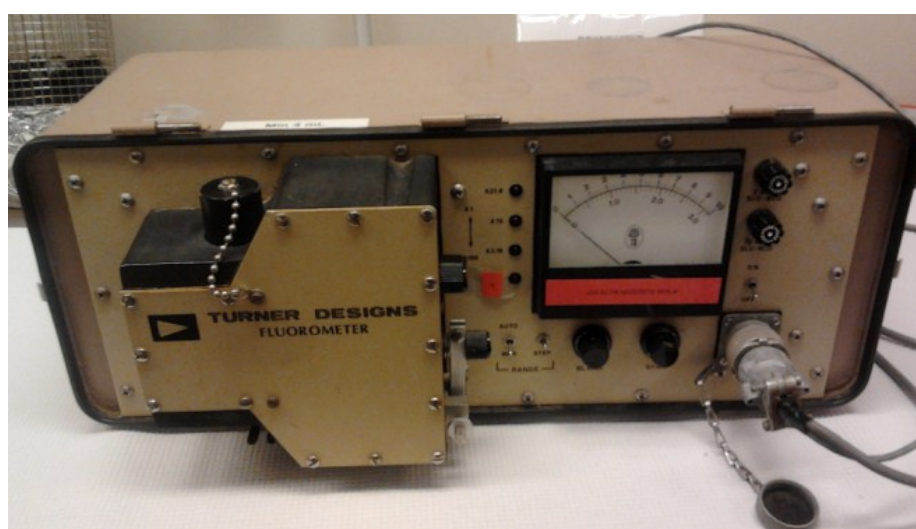
Figure 9 The overview of fluorometer (10AU™ Field and Laboratory Fluorometer, TURNER DESIGNS, USA). (Photo by Xixi LIU)
