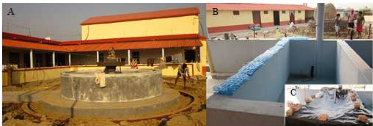
Figure 8: Working site with experimental tanks exposed to natural outdoor light conditions (A,B), and covered up with black plastic to simulate extended darkness (C).
