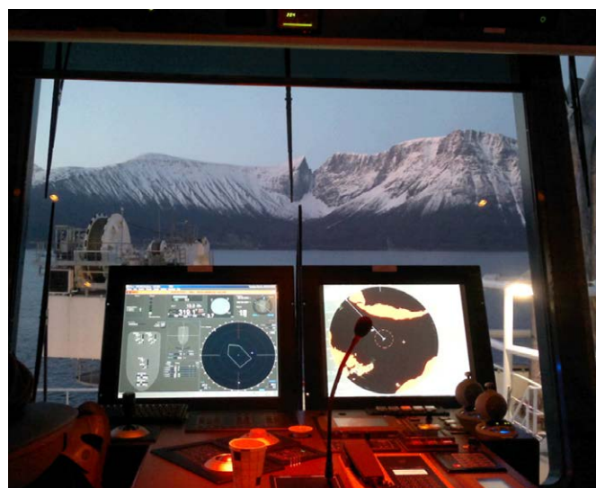
Fig. 23. Picture taken by the first author at a sea trial in a Norwegian fjord in April 2012 onboard a multi-purpose offshore vessel with 5 thrusters (11 MW) and K-Pos DP21.
