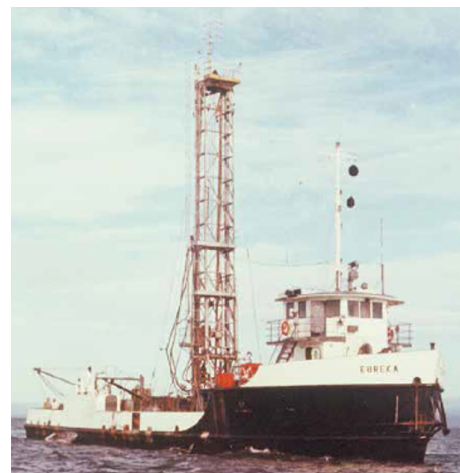
Fig. 2. The Eureka (1961) was the world’s first automatically positioned vessel. Picture courtesy of Howard Shatto.
