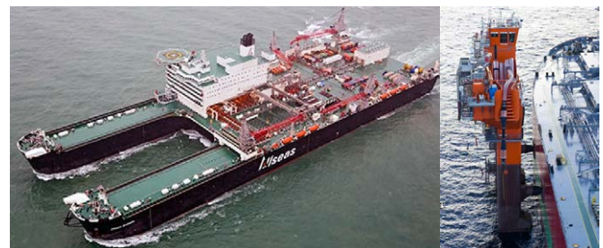
Fig. 22. Left: The ocean giant Pioneering Spirit. Picture courtesy of Allseas. Right: The HiLoad "clamp-on DP" unit. Picture courtesy of Remora.
