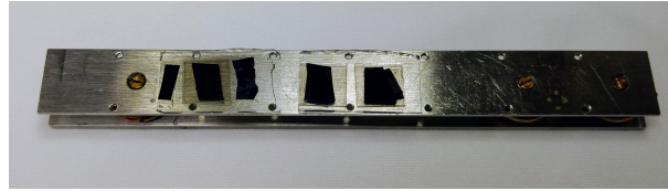
Figure 4.4: Three STO substrates mounted on a holder, ready for XPS. The substrates are attached with carbon tape (black) to glass plates, which in turn are attached to the sample holder with carbon tape.
