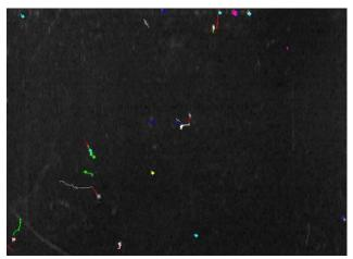
Figure 5. Screenshot from ImageJ with the particle tracker. The coloured dots and lines are detected particles and their trajectory.
