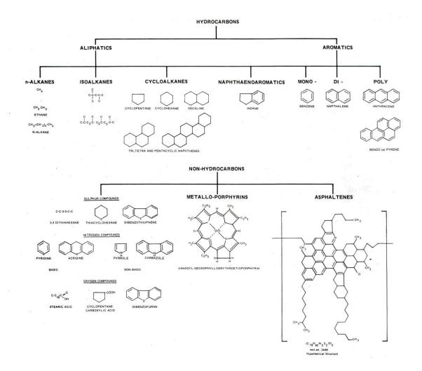
Figure 1. Some of the common hydrocarbons and non-hydrocarbons present in crude oil(Miller and Connell, 1982).
