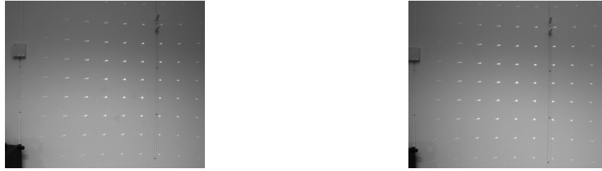
Figure 2.27: Structured light on wall, as seen from the left and right camera.
