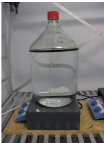
Figure 4: Setup for making WSF from Troll B fresh crude oil. A stirring magnet at the bottom of the flask enhance equilibrium between the oil components dissolved in the water and the crude oil. The glass tube inside the bottle is used for tapping of the WSF after the stirring is finished. The whole system is closed with a Teflon-lined cap.
