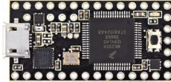
FIGURE 3.8: The Teensy 3.1 Microcontroller Unit used for both the Pixcuckoo and the Tracker. Read Appendix A for more detailed information about the Teensy 3.1 MCU and its Cortex M4 Microprocessor.
