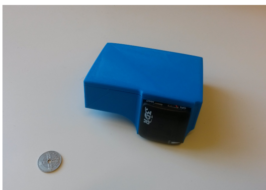
(A) Tracker prototype with lid in place, protecting to the sensitive electronics inside.
