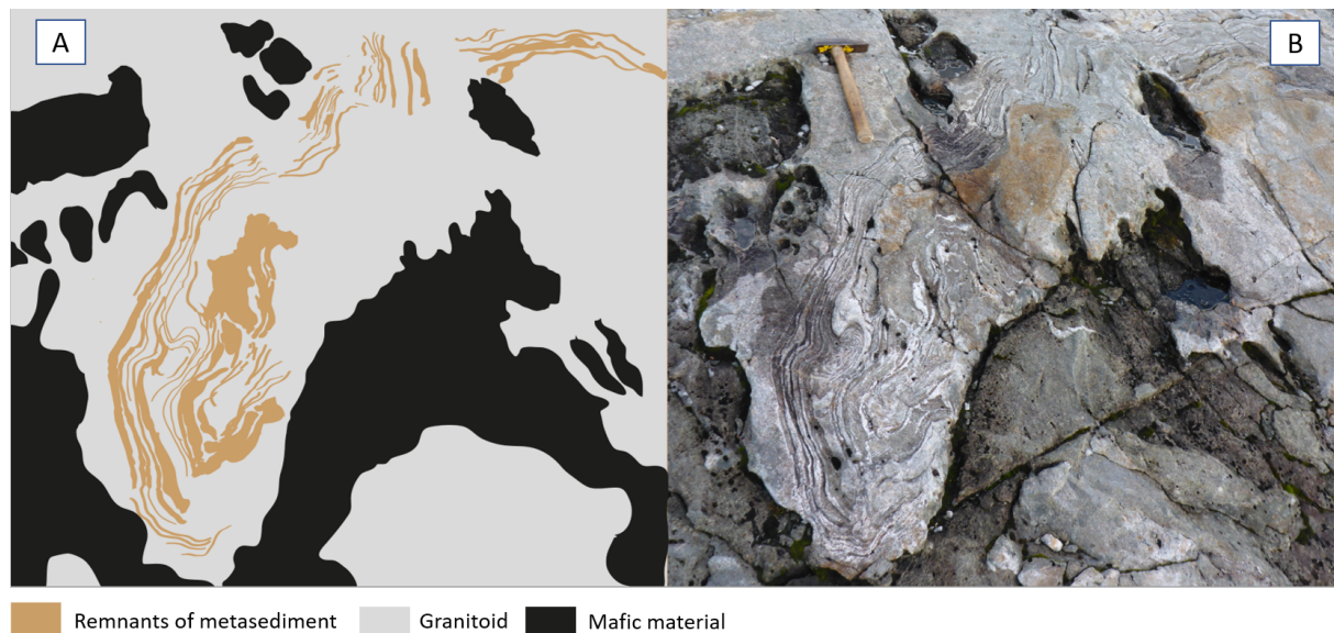
Figure 5.8: A) Sketch displaying the interaction between various lithologic units in the the contact zone. Remnants of metasediments are dislocated and randomly distributed within the granitoid. Irregular mafic enclaves of various size are enclosed in the granitoid. There are internal variations in the abundance of dark minerals in the contact granitoid, which is not displayed in this simplified sketch. B) Picture of the locality which the sketch is based on, with a hammer for scale. Picture was taken a few 100 m north of Austre Sauvatnet.
