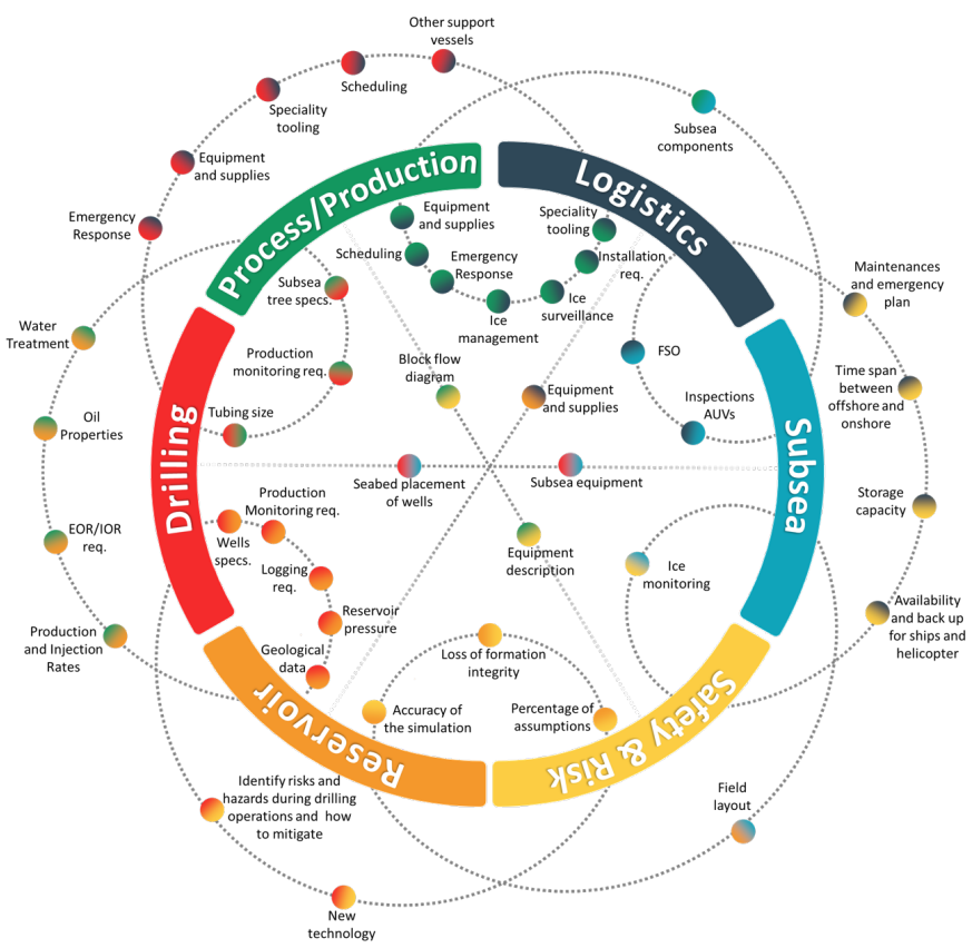
Figure 2.7: Boundary chart of the information that has to be conveyed in a typical field development project
