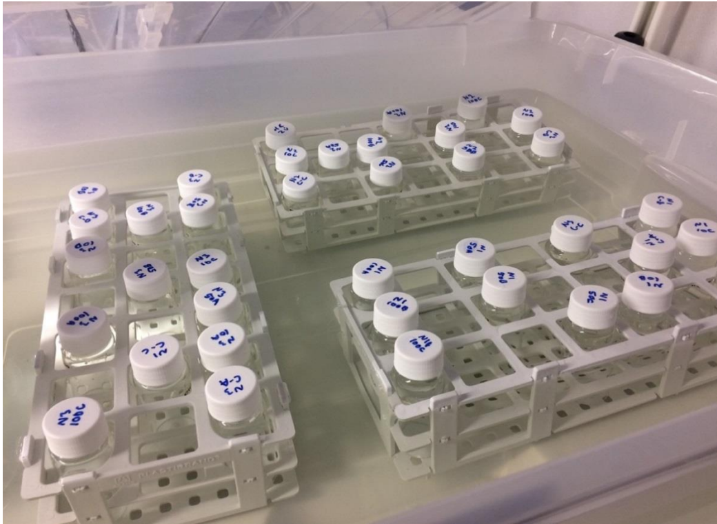
Figure 3.2 Experimental setup for rearing of C. finmarchicus and C. hyperboreus exposed to WSF at different temperatures. The experiments were conducted in glass vials, marked with corresponding exposure and life stage, placed in racks immersed in water baths to decrease temperature variations.
