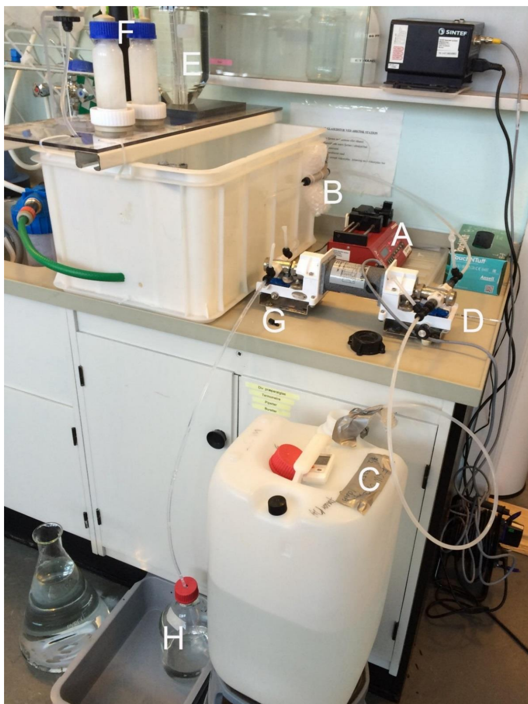
Figure 3.3 Setup of the water soluble fraction generation system. N-alkane oil spiked with 11 selected PAHs was pumped from a glass syringe (A) to the droplet generator (B) where it was forced together with filtered seawater (C) pumped at a flowrate of 160 \text{ mL min}^{-1} (D), generating a dispersion. The dispersion was kept in the overflow chamber (E) to provide sufficient residence time to assume equilibrium between the PAHs dissolved in the water and in the oil droplets. The dispersion was sucked through two parallel filter units (F) by a pump with a flowrate of 140 \text{ mL min}^{-1} (G) to ensure only the WSF (H) to come through.
