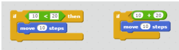
Figure 2.5: Two attempts at creating an if-statement in Scratch. The one on the right remains disconnected due to incompatible blocks
