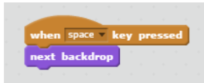
Figure 2.6: An event handler that changes to the next backdrop when the space bar is pressed
