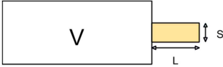
Figure 3.2 – The Helmholtz resonator as an acoustical mass-spring system.
