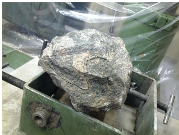
Figure 4.7: Picture of rock sample collected in Hammerfest. The rock show banding and distinct folding patterns.
