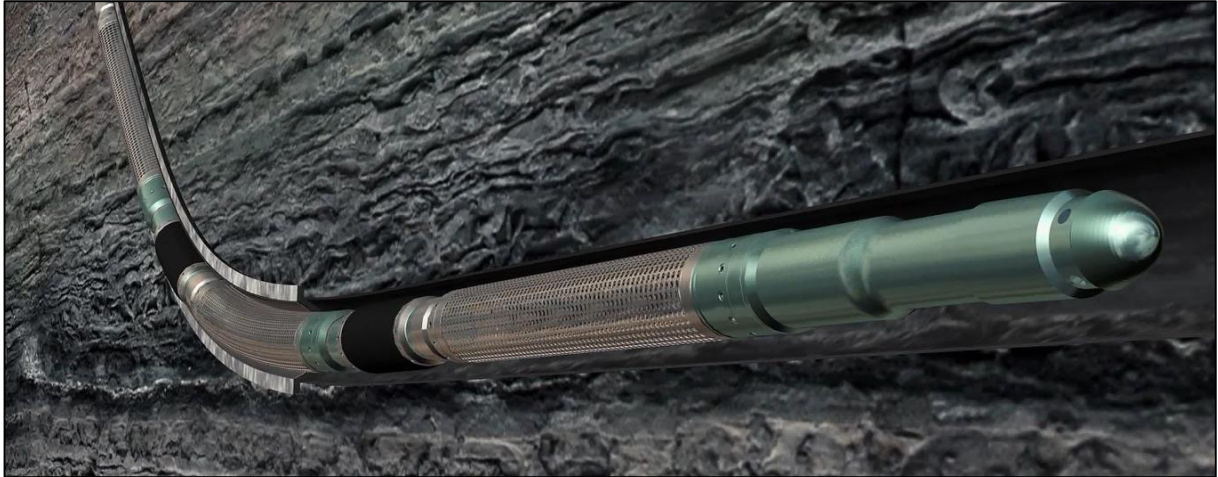
Figure 4-2: Snap Shot of Reamer Shoe and Sand Screens Downhole (Screenshot from Ridge AS Animation, 2016)
