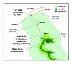
Figure 3.5: Ice management fields and ice drift (Fenz et. al 2013)
