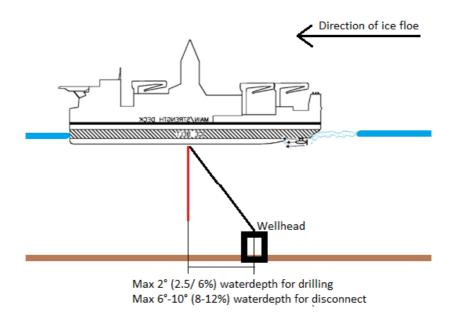
Figure 3.2: Stationkeeping and Anchoring
