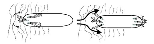
Figure 3.1: Thrusters pushing sea ice out from hull, and counteracting to maintain position (Statoil 2013)
