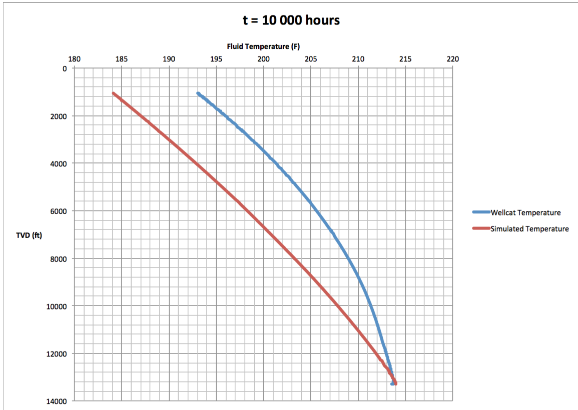
Figure 5-10 Fluid Temperatures, t=10 000 hours
