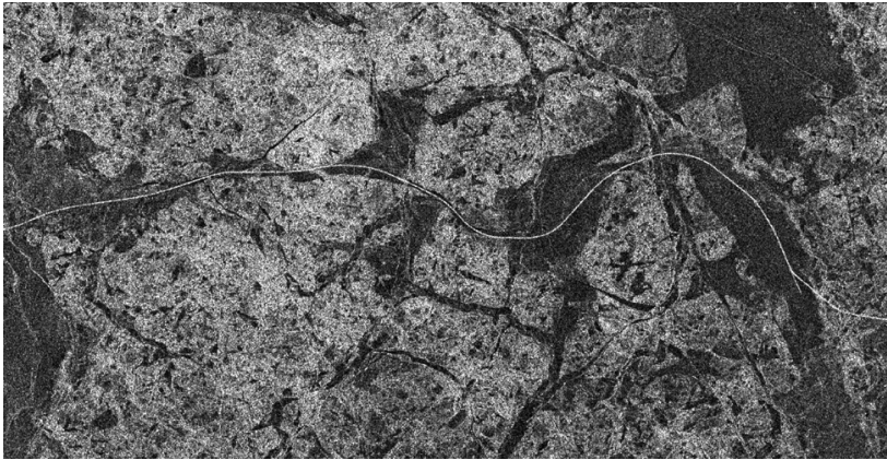
Figure 3.3: Part of an ERS-2 SAR scene from 6 May 1998, the bright line is the strong return signal of the ship track through the level sea ice areas in the Ob Estuary. The image size is 16 by 31 km. Image Data ©European Space Agency/Nansen Environmental and Remote Sensing Center 1998.
