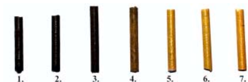
Figure B-2: Samples saturated with \text{CuO} taken at 1020 °C from melts with 1) Natural cryolite, 2) 0.7 wt% alumina, 3) 1.25 wt% alumina, 4) 2.5 wt% alumina, 5) 5.0 wt% alumina, 6) 6.0 wt% alumina, and 7) 10.0 wt% alumina added to natural cryolite melts.
