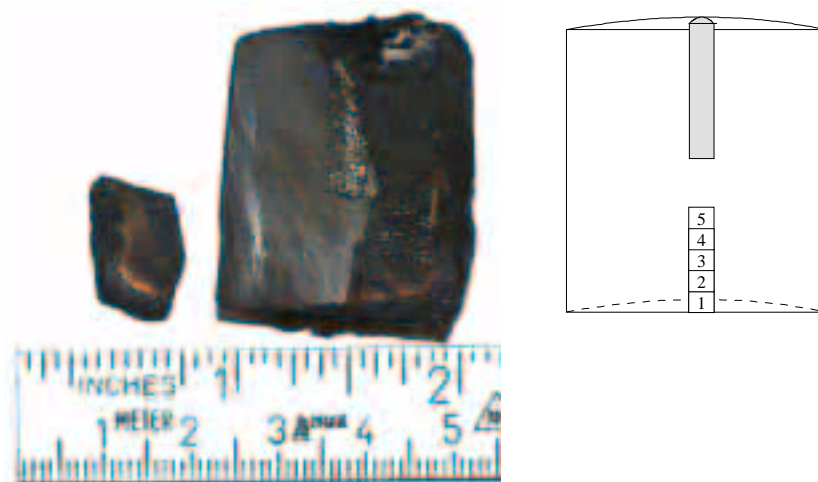
Figure 7-11: Picture showing the interior of a cermet anode (with 17% excess NiO, 17% Cu and 3% Ni prior to sintering) cut into two pieces after 22 hours of electrolysis in alumina saturated melt with CR = 2.29, T = 960 °C and 1 \text{ A/cm}^2 . The numbered squares in the sketch of the anode illustrate which part of the anode that was analysed by element mapping Figure 7-12 shows the mapping labelled number 1.
