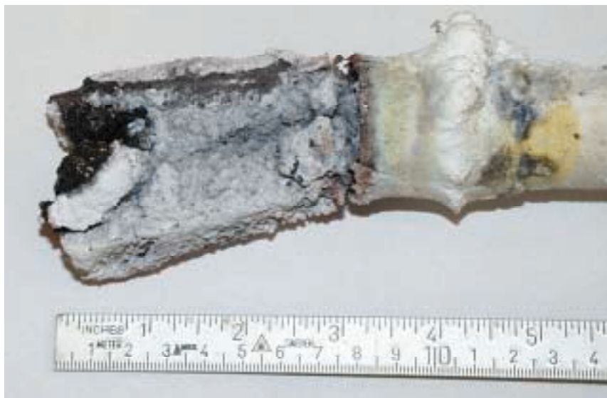
Figure 7-7: Growth on a TiB 2 cathode after 48 hours of electrolysis. The cathode shown was suspended 90° counter-clockwise in the electrolysis cell.
