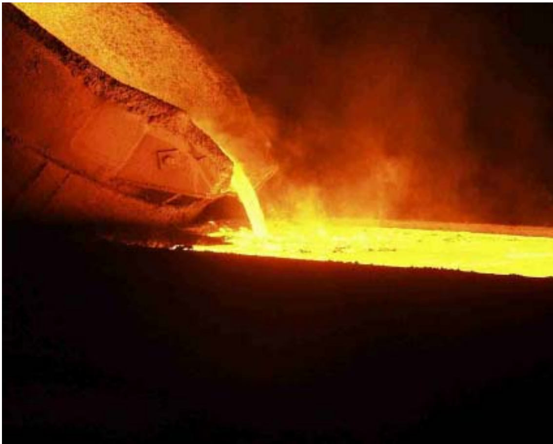
Figure 1.1 Photograph taken during casting of ferrosilicon from ladle to open mould. Elkem Thamshavn, Norway, 2000.
