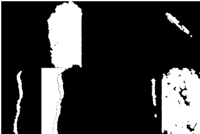
Figure 4. Y-image mask of (0/1) discrimination areas. Note that by using a relevant background discrimination feature, it is possible to zoom in only on the true flaws present in the gridded calibration imagery, which have been designated white here.
