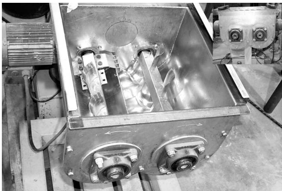
Figure 12.The IDE-CON continuous mixer. Note the two counter-rotating shovels of the new, proprietary IDE-CON design.
