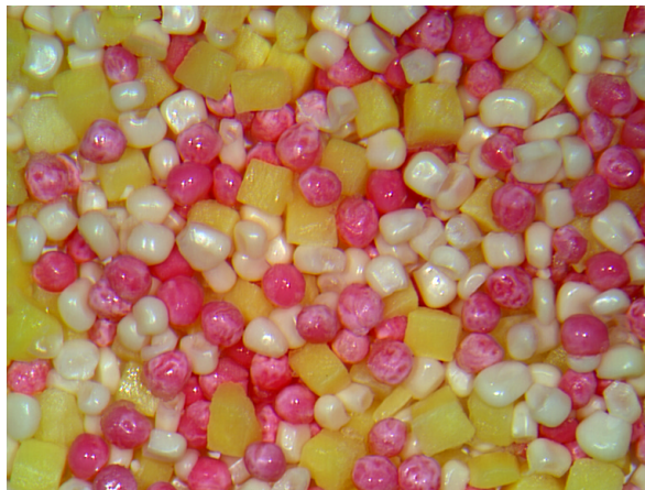
Figure 18. RAW image of a three-component mix in NIR, Red and Green channels
