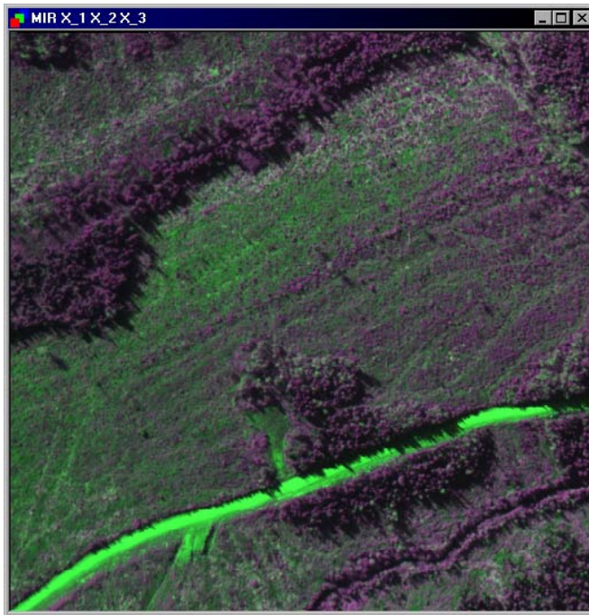
Figure 1. The scene space master image data which will be used for illustration, the Montmorency Forest data set [7,8]. The image consists of 512x512 pixels in eight bands (Channels, variables). Here it is represented by channels 1-2-3 as R-G-B.
