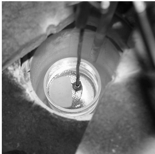
Figure 6.5: Tablet agglomerate in place just below the melt surface. The tablet suspension rig is a steel wire mesh fixed at the end of a 3 mm k-type thermocouple.
