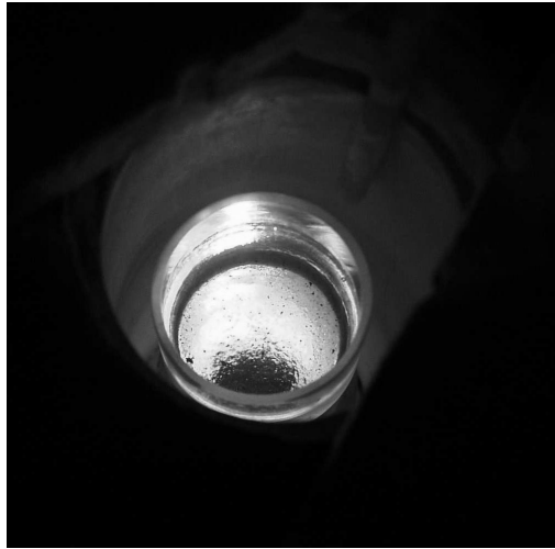
Figure 6.4: View of quartz crucible with melt seen from above. The rough surface that has developed on the crucible bottom after melt-down is evidently of the order of \sim 1 mm. Under-exposed image due to intense light source from below.
