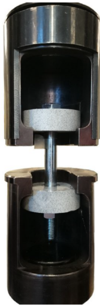
a) Photo of a bolt mounted in the purpose-made grips
