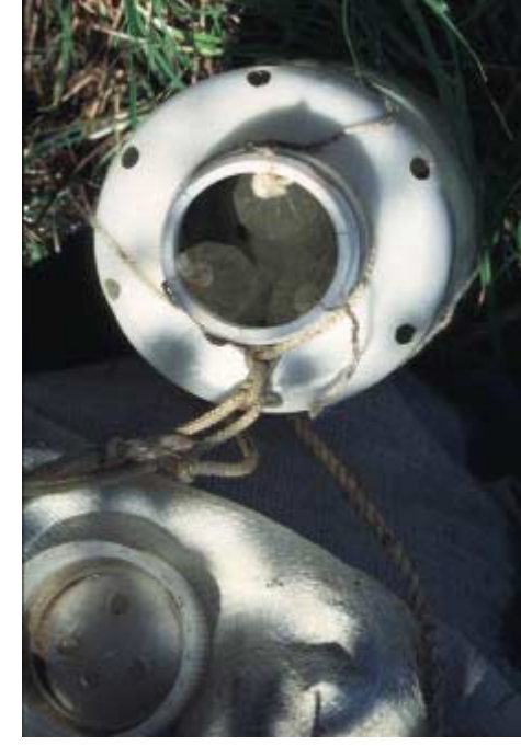
Figure P.28: Drilled holes on the top and bottom of the protecting bottle ensured that water could flow through. Thin wires were tied to one end of the bags, and a knot was made on this wire ~2 cm over the bag. After having collected the old dialysis
