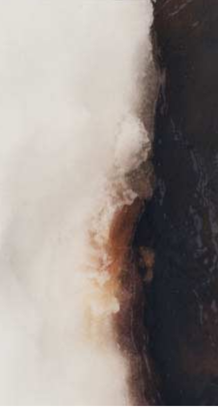
Figure P.23: The lower 20 cm of the snow-cap covering river Orva were completely red and extremely up-concentrated on Cu compared to the river water.
