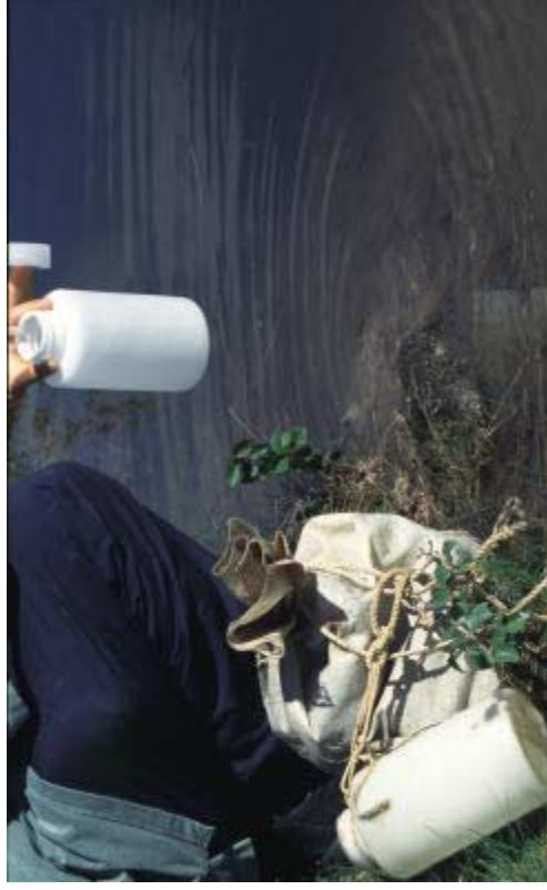
Figure P.27: The (left) plastic bottle that protected the dialysis bag in the river was tied to a stone-filled potato bag connected to land with a rope.
