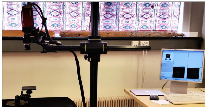
Figure 4.1: Configuration of ATOS III SO at the Department of Structural Engineering.
