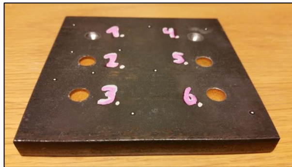
Figure 4.8: Artificial corrosion pits
