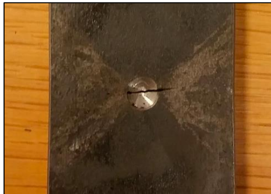
Figure 5.4: Partial failure of pit 3 in specimen 1
