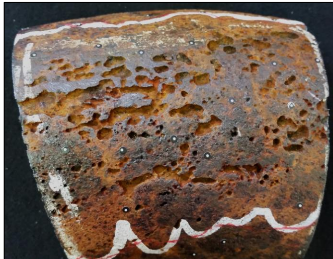
Figure 4.12: Example of chain section with corrosion pits (courtesy Statoil ASA)
