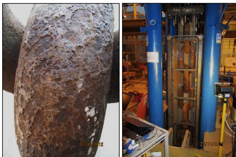
Figure 5.7: Chain from Åsgard A (left) and testing rig (right). (Fredheim et al. (2013), p. 3 and 6)
