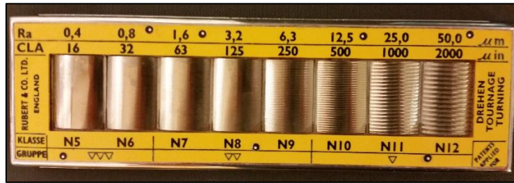
Figure 4.10: Surface roughness specimen
