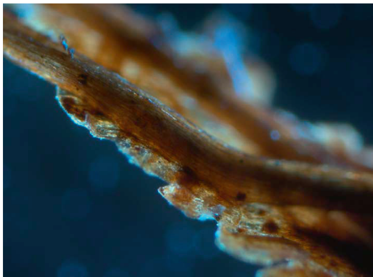
Fig 1. Microscopic image of a sample indicating the wood and the amorphous organic substance that is strongly adhered to the wood. The organic deposit is observed as dark brown amorphous encrustation under microscope. From the visual examinations under normal and polarized light, the amorphous organic substance appears as a brownish tar-like material. In its appearance it also looks homogeneous to some extent.
