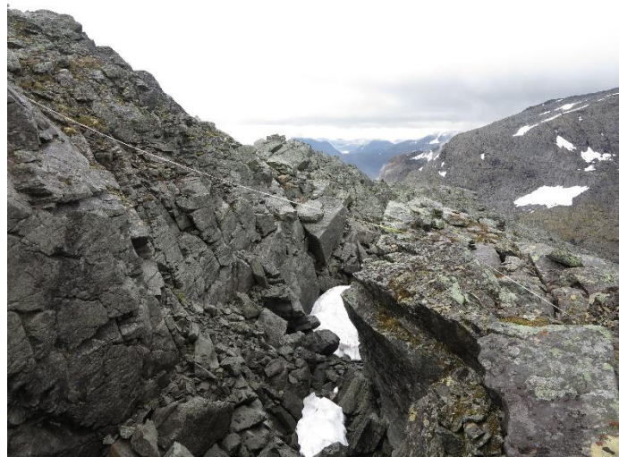
Figure 5.2 Photo showing the thickness vs. shortest axis ratio of the blocks along the main scanline in the source area. Unfortunately, the photo does not have any scale, but the open crack is measured to be 4.5 m wide.
