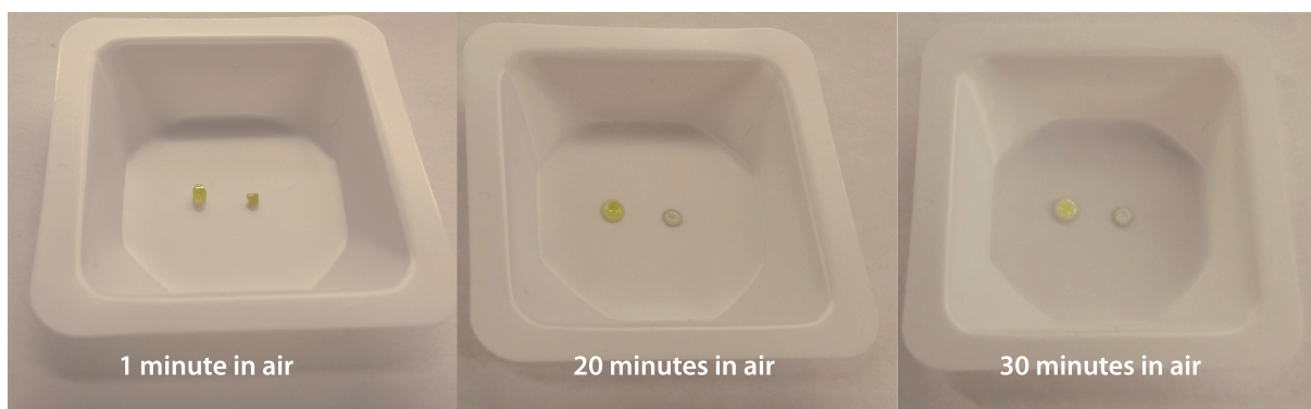
Figure 2.13: Illustration of Rhenium(VII)oxide, \text{Re}_2\text{O}_7 , hygroscopic nature. The image shows crystals exposed to air for 1, 20 and 30 minutes.
