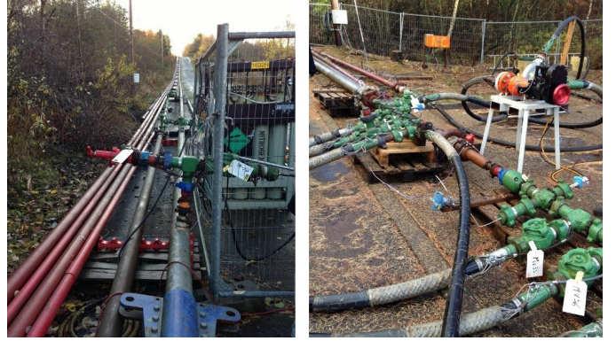
Fig. 2. Flow loop with drillstring washout and gas injection (left), and fluid loss and drill bit (right).
