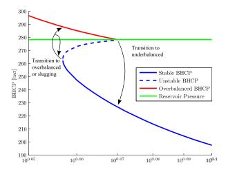
Fig. 2. Equilibrium values of the BHCP with respect to valve opening. For each value of the valve opening, there is at most 3 potential operating points [Aarsnes et al., 2014a].
