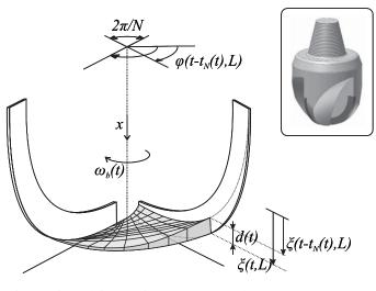
Fig. 3. Bit-rock interaction [Germay et al., 2009].
