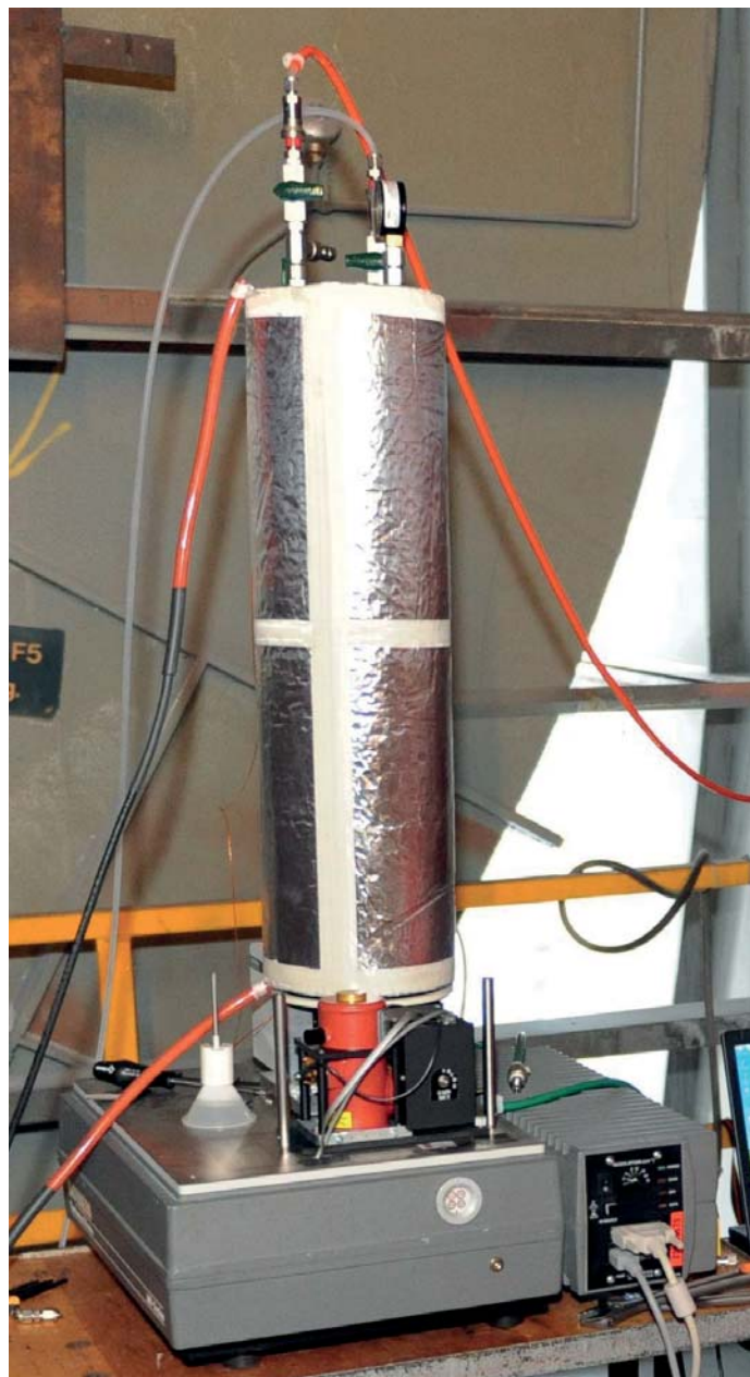
Figure 3.1: Apparatus setup with Bomem FTIR, a liquid N 2 cooled MCT detector and a large 11 L / 35 m cell. Two connected heat elements are covering the cell. Nitrogen is continuously flushed between the detector housings and the cell. (MCT detector housing detached in picture. During operation it covers the red N 2 cylinder and black detector box.)
