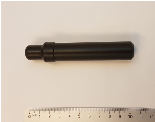
Figure 4.2: The acoustic emitter used in the experiment. One of the largest emitters produced by Thelma Biotel customized with a static 7 second transmission interval.
