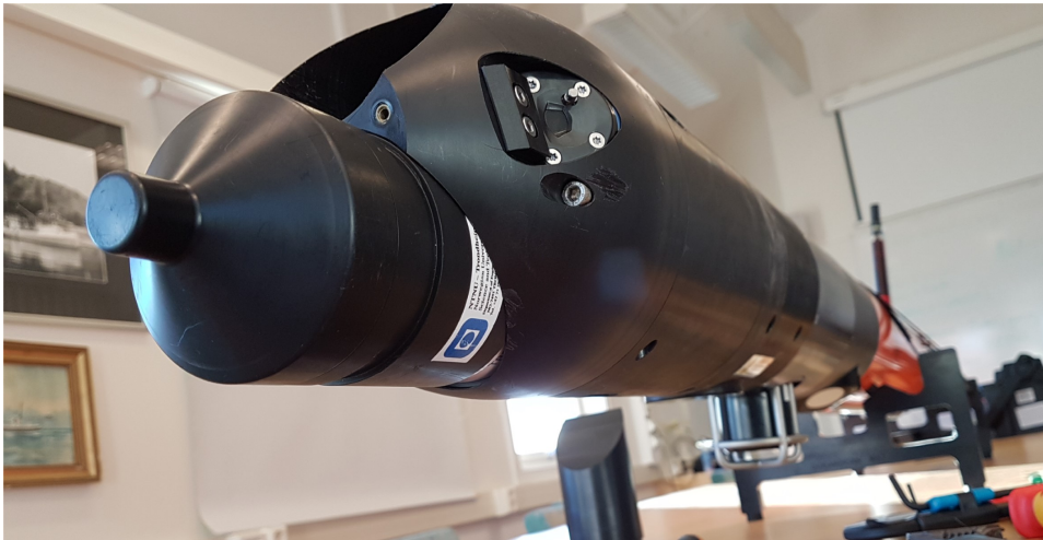
Figure 5.5: Hydrophone successfully mounted and connected in the wet section
