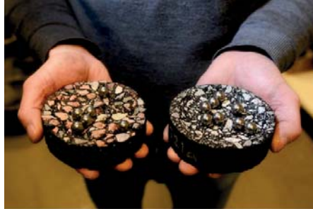
Figure 11: Prall Test specimens after the test with some of the steel spheres (Photo by Knut Opeide)
