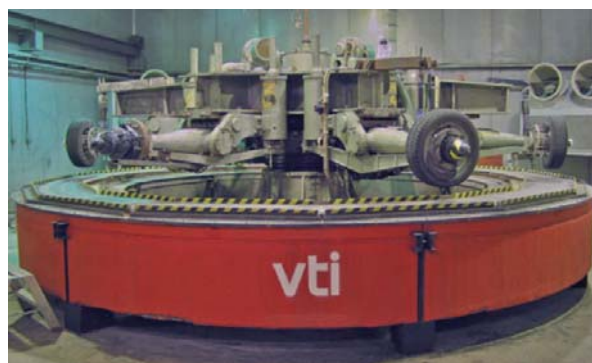
Figure 13: Road Simulator (Photo by VTI)
