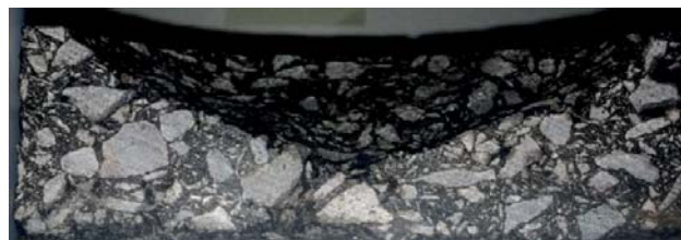
Figure 6: Cut specimen of AC8A after testing with the Prall Test
