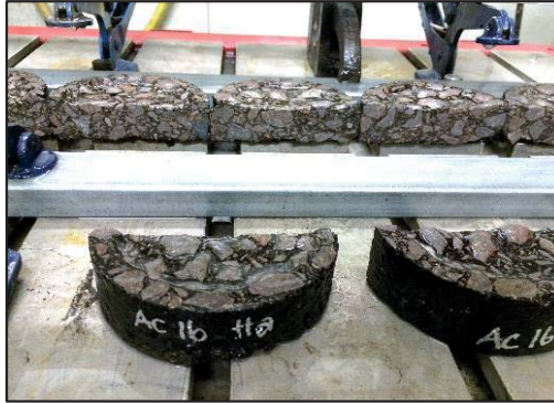
Figure 3: Cut Prall Test specimens
