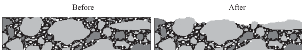
Figure 1: Pavement surface before and after exposure to studded tires
