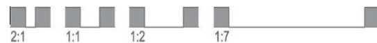
Figure 10. Proportion between heights of blocks and width of the street in relation to the 1:1 ratio, picture: Author.
