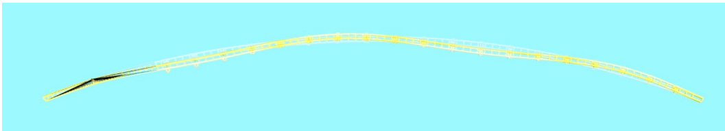
Figure 5.3: Eigenmode with eigenperiod of 20.76 seconds
