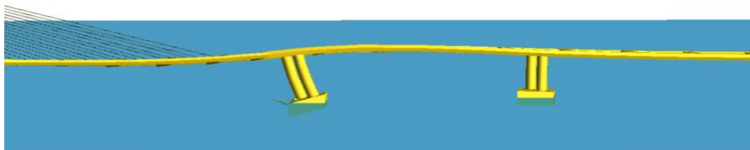
Figure 7.26: Deformation of bridge after 21.83 seconds, showing a local bedding of the bridge girder, due to pendulum motion of the pontoon. Deformations scaled by a factor of 10
