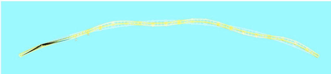
Figure 10.9: Eigenmode with eigenperiod of 11.02 seconds
