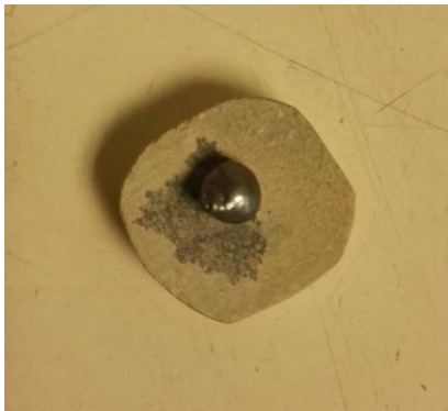
Figure 4.3: Photo of a sessile drop on coated \text{Si}_3\text{N}_4 sample substrate.
