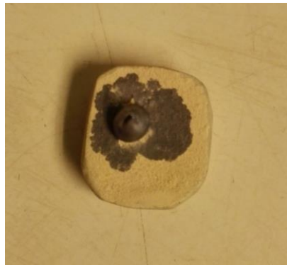
Figure 4.1: Photo of a sessile drop on uncoated \text{Si}_3\text{N}_4 sample substrate.
