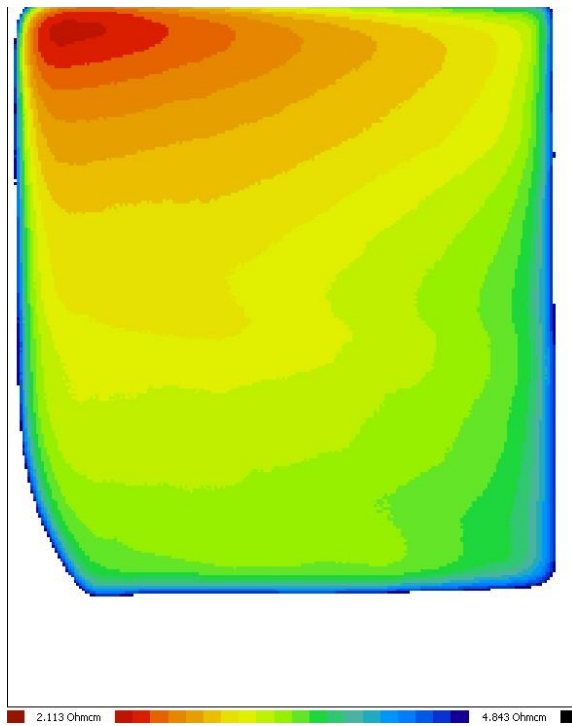
Figure 4.22: Mapping of resistivity in IC4 by eddy currents.
