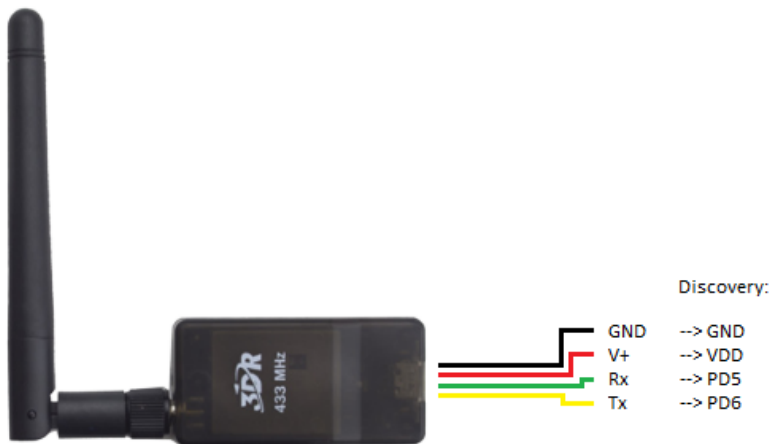
Figure 6.12: Pinout 3DR Radio Telemetry Kit
