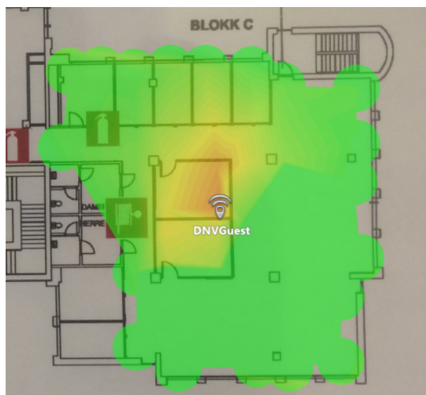
Figure 5.6: Improved Coverage Block C. Dark blue indicates signal strengths weaker than -67 dbm
