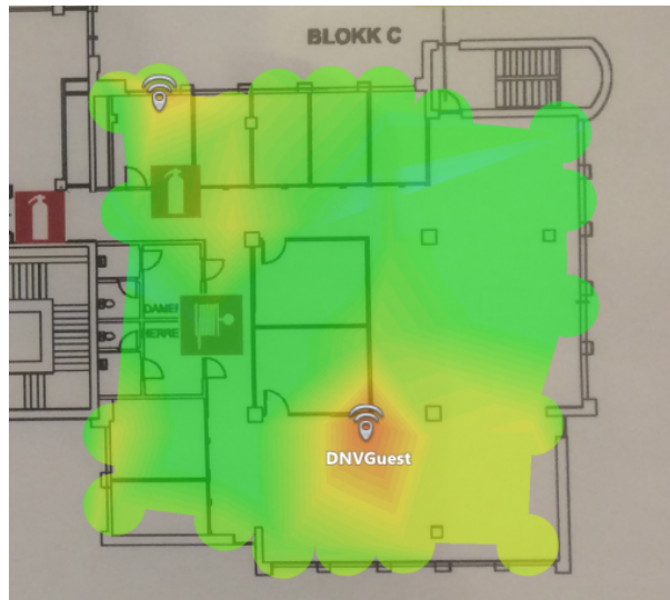
Figure 5.7: Additional AP placed in Block C. Dark blue indicates signal strengths weaker than -67 dbm
