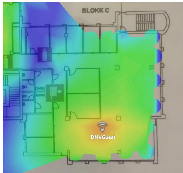
Figure 5.5: Initial coverage Block C. Dark blue indicates signal strengths weaker than -67 dbm
