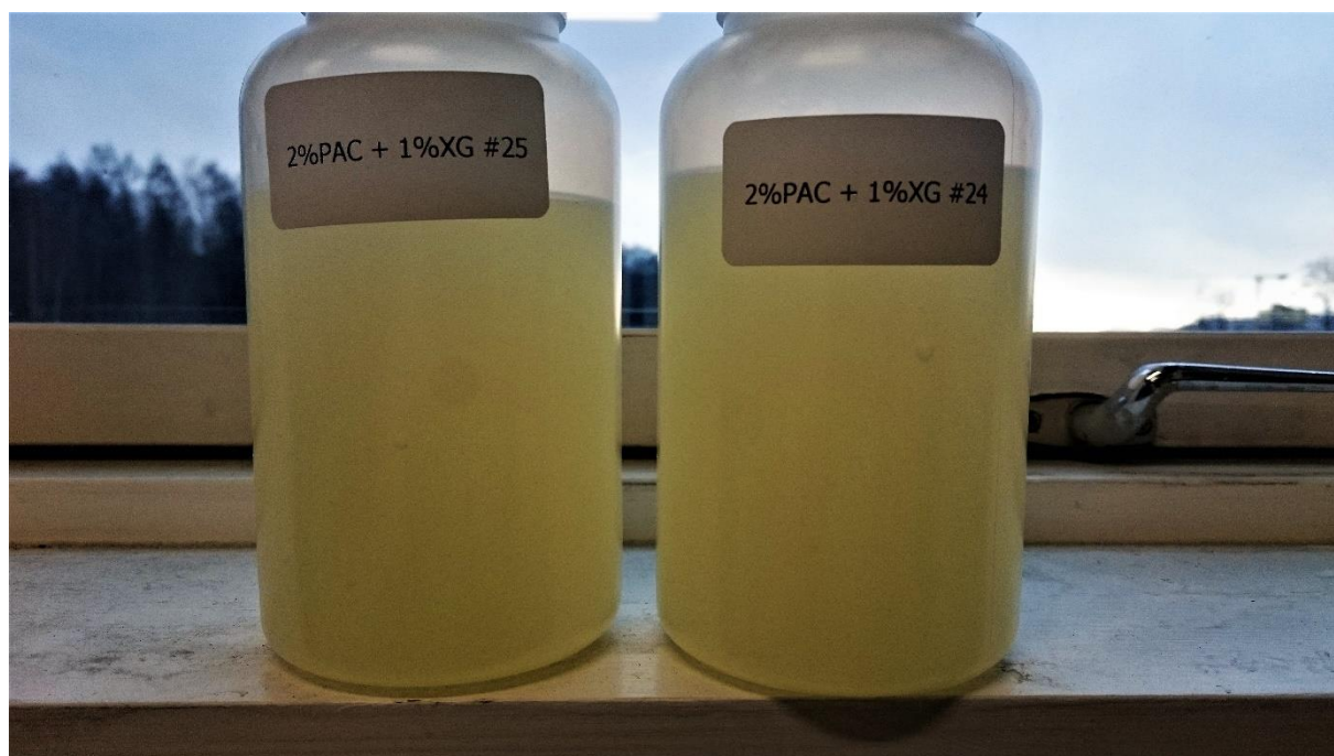
Figure 45: Gasification after 72 hours, 2% PAC+1%XG
