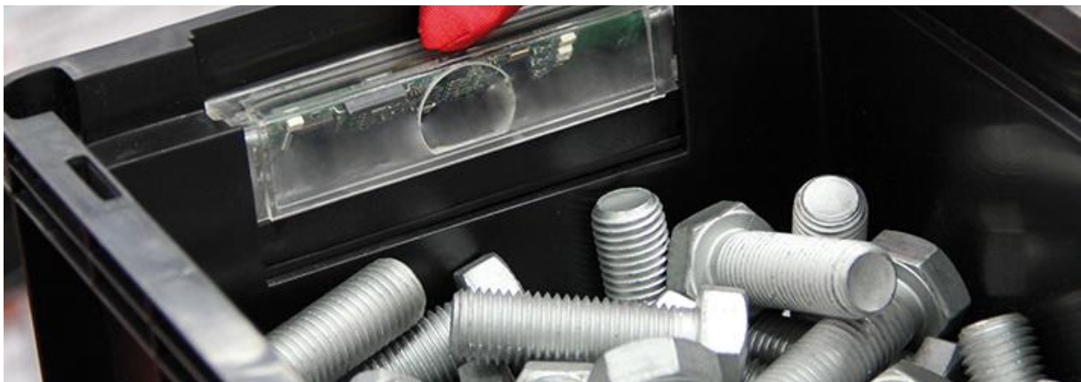
Figure 19 Illustration of iBin container with optics (Würth Industrie, 2016)
