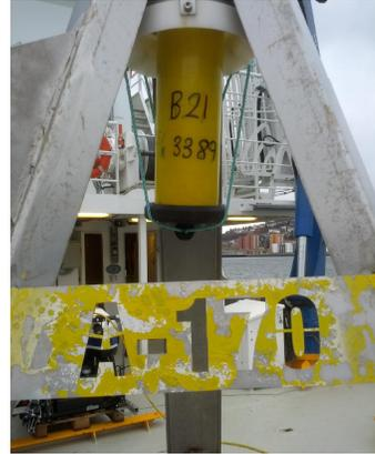
(b) Transponder attached to tripod forming a transponder tower [3]. The tower carries one of four transponders in the LBL network deployed outside TBS in 2013 [3]. The transponders are located 250 and 400 meters away from land.
