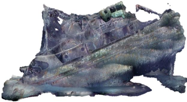
(a) 3D model of the Herkules wreck produced from the stereo system. Herkules is a tug that sank in 1957 due to poor seamanship [1]. The wreck is what divers call a Donald Duck wreck; a rather intact wreck standing on the keel.
