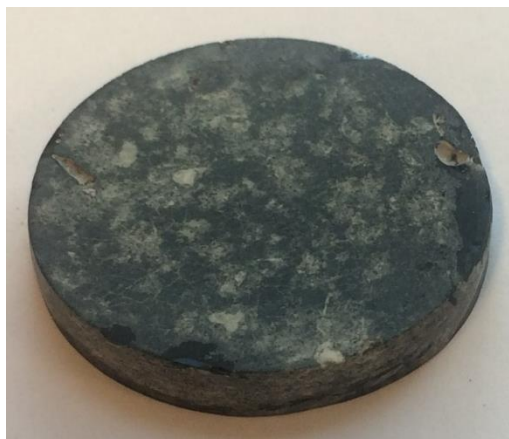
Figure 11.5: Specimen AD-02 (box 12) with irregularities corrected with epoxy (dark regions on the specimen edges).
