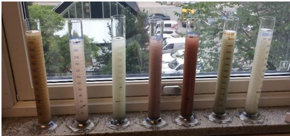
Figure 6.B.2: Measuring cylinders with fine-fraction material dissolved in water
