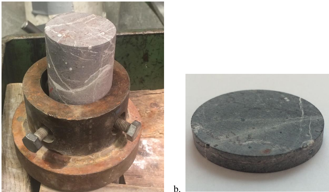
Figure 11.3 a) Sample AQD-02 (box 12) ready to be prepared b) Preparation completed.
