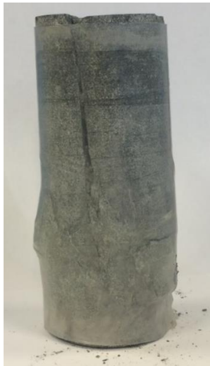
Figure 8.1 Axial splitting of AD-02 (box 8)
