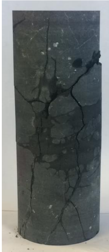
Figure 8.3 Complex fracturing of sample AQD-02 (box 8)
